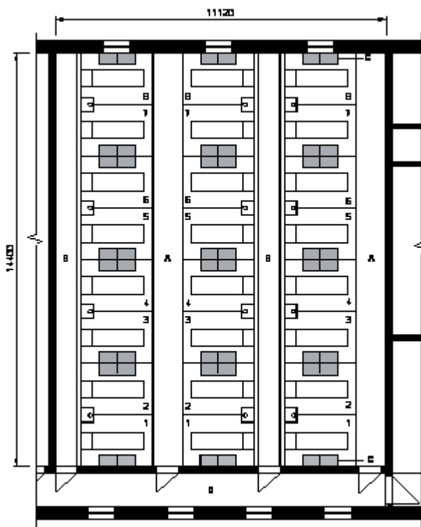
Fig. 1: Layout of the 1 st farrowing section (from the total number of 5) with 3 x 8 farrowing pens with crate and warm-water pads for floor heating of piglets
